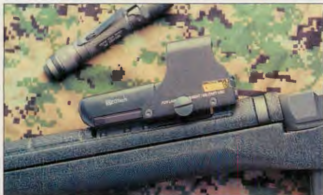
Here the Eotech red reticle sight is mounted on the forward rail of the SOCOM 16.
